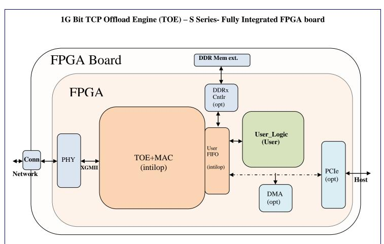
FPGA Board System with fully integrated and tested; PHY+MAC+TOE+Host\_IF, available on select boards from intilop board partners
